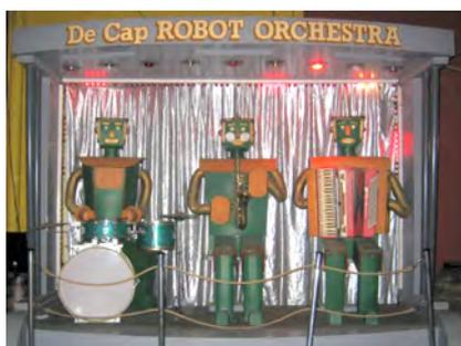
The De Cap Robot Orchestra, a 105 key organ built in the early 1950s. The onstage life size robots have different facial expressions and play saxophone, percussion and accordion. Their automation consists of at least 20 movements, including eyes, fingers, feet, hands and head, and is accompanied by a synchronised light show. Its original location was Scotland.
